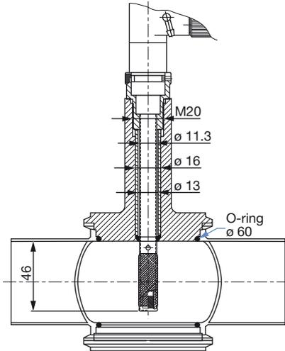
with adaptation set Clamp 2" external  $\phi$  64 mm
