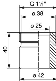
Blind plug for welding tab DN30
