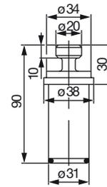
Nut for blind plug (welding tab DN30)
